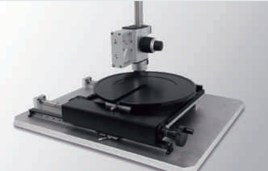
A stand that allows you to observe a disk-shaped object from the edge to the center while rotating it. Compatible with 12 inch wafers.
